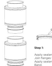
Apply sealant to flange surface. Join flanges together. Apply sealant to the inner groove of the V-Band. Position V-Band around the flanges and tighten.
