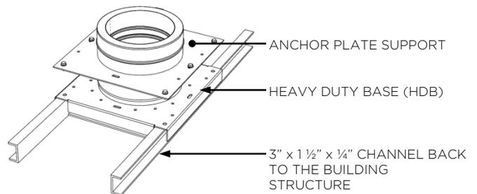
Figure 2-6, Heavy Duty Based Support for Horizontal
