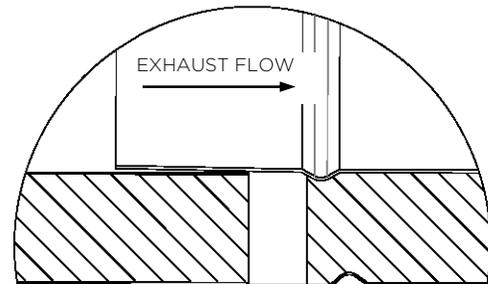
CUT END STARTS TO ENGAGE AT 1.2" INTO OTHER PIPE.
