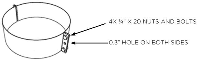
Figure 2-14, Light Support Band Installation Example
