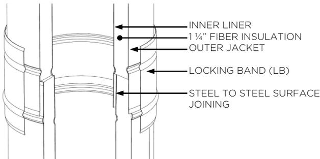
Further features of Model DWKL double wall and fiber insulated include:
