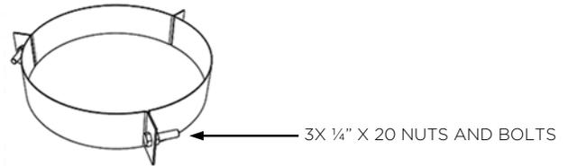
Figure 2-16, Guy Wire Band Installation Example
