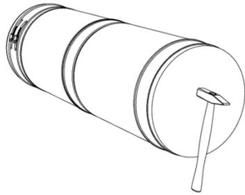
Tap 2-3 times. Make sure to press both inner and outer pipes together; the inner should not be more than 1/8" longer than the outer pipe once the male/female conical ends are engaged.
