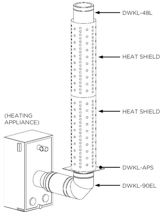
Figure 6-8, Horizontal Installation Example
