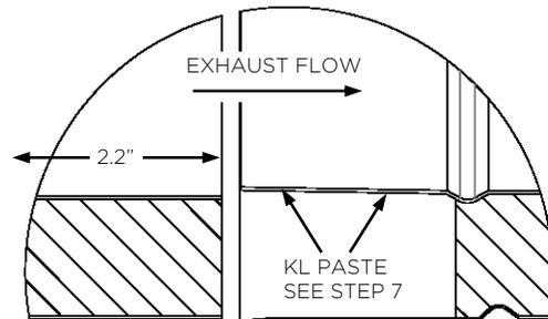
MARK 2.2" FROM THE END OF CUT BEFORE BEING INSERTED INTO THE CONNECTING PIPE CONICAL INLET.
