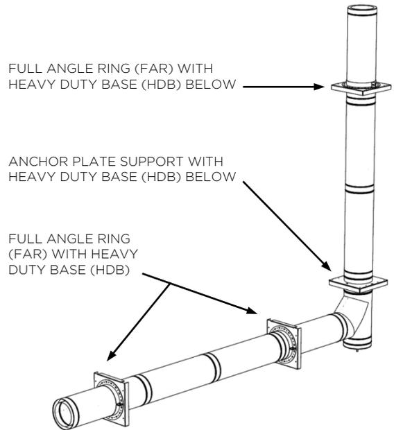
Figure 2-11, Wall Brackets for Full Angle Ring Example
