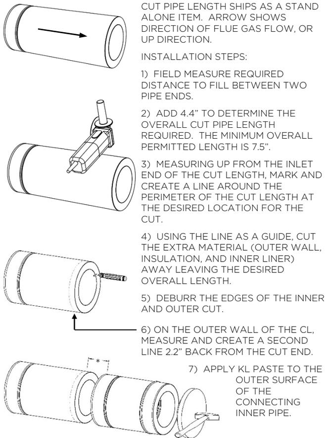
8) TAP THE ADJOINING LENGTH OR CUT LENGTH INTO PLACE USING THE SUPPLIED WOOD PLATE. PROPER ENGAGEMENT IS ACHIEVED WHEN THIS DIMENSION (\*) BECOMES ZERO.
