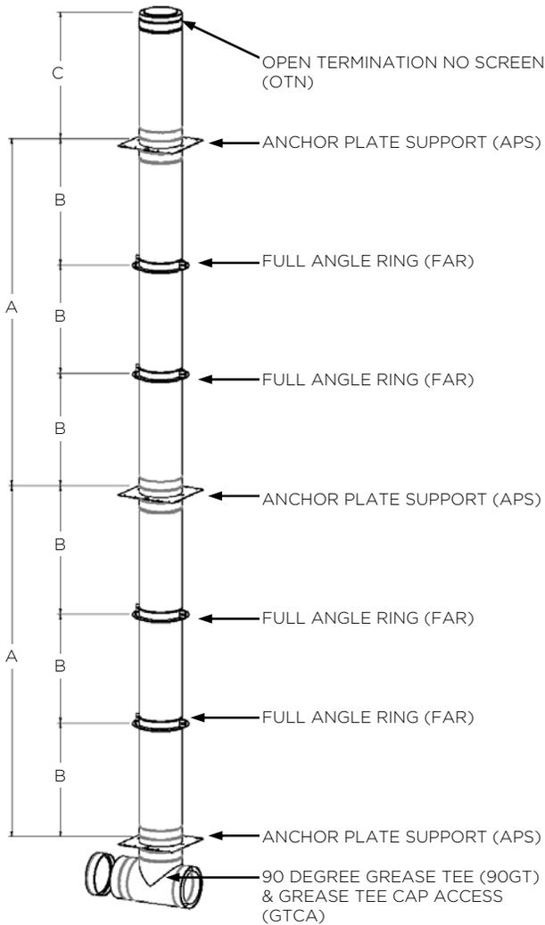
NOTE: See PART 3 "Lengths for Thermal Expansion" in these instructions for important use of expansion joints between anchor plate support locations.
