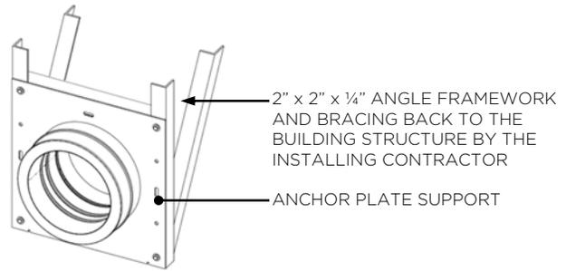
The Anchor Plate Support may only be attached to non-combustible construction such as block, concrete, or steel.
