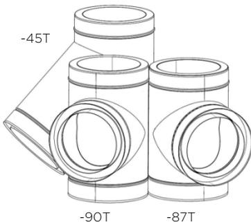
Figure 4-6, 45°, 87°, & 90° Grease Duct Boot Tee
