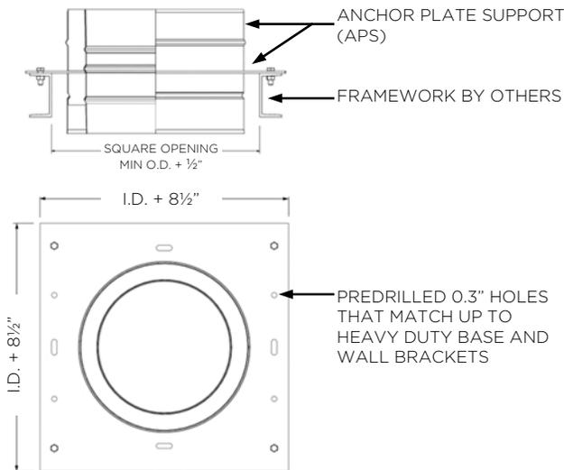
The plate must be braced back to the building structure or support with rigid structural members by the installing contractor. The structural project engineer should select support members in accordance with good engineering practice to suit each specific application, or follow the guidelines to meet the following figures.
