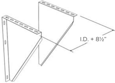
Hardware for attaching the Anchor Plate Support to the Wall Brackets is supplied with the brackets.
