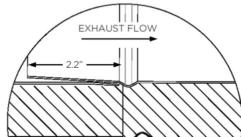
CUT END IS FULLY ENGAGED (2.2") BY TAPPING THE PIPES TOGETHER UNTIL THE OUTLET END OF THE CUT LENGTH IS FULLY ENGAGED (CREATING A TIGHT SEAL) INTO THE CONICAL INLET OF THE CONNECTING PIPE. FOR DWKL THIS OCCURS WHEN THE OUTER WALL OF THE CONNECTING PIPE ENGAGES TO THE CUT LENGTH OUTER WALL LINE CREATED IN STEP 6.
