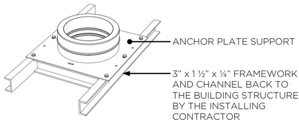
Figure 2-4, Anchor Plate Support for Horizontal
